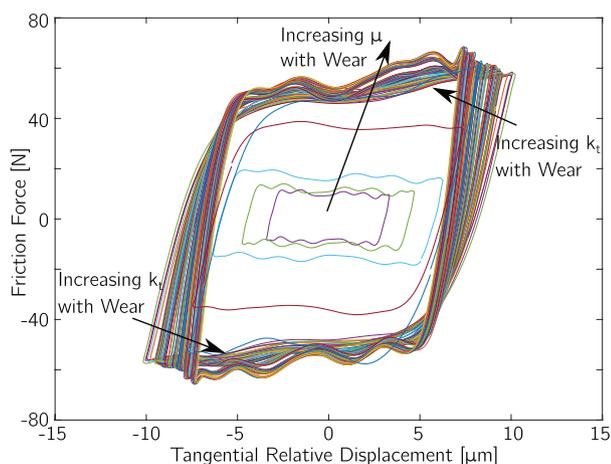
Fig. 4. Evolution of hysteresis loops with wear for test 1: excitation frequency = 100 Hz, average sliding distance =  $\pm 7\mu\text{m}$ , normal load = 60 N, nominal area of contact =  $1\text{mm}^2$ , total fretting cycles = 1900000, material = Stainless Steel, temperature = 25° C.
