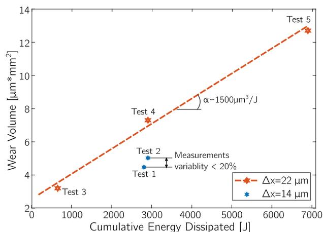
Fig. 7. Wear volume as a function of energy dissipated at the contact. Test conditions: excitation frequency = 100 Hz, normal load = 60 N, nominal area of contact =  $1\text{mm}^2$ , material = Stainless Steel, temperature =  $25^\circ\text{C}$ .
