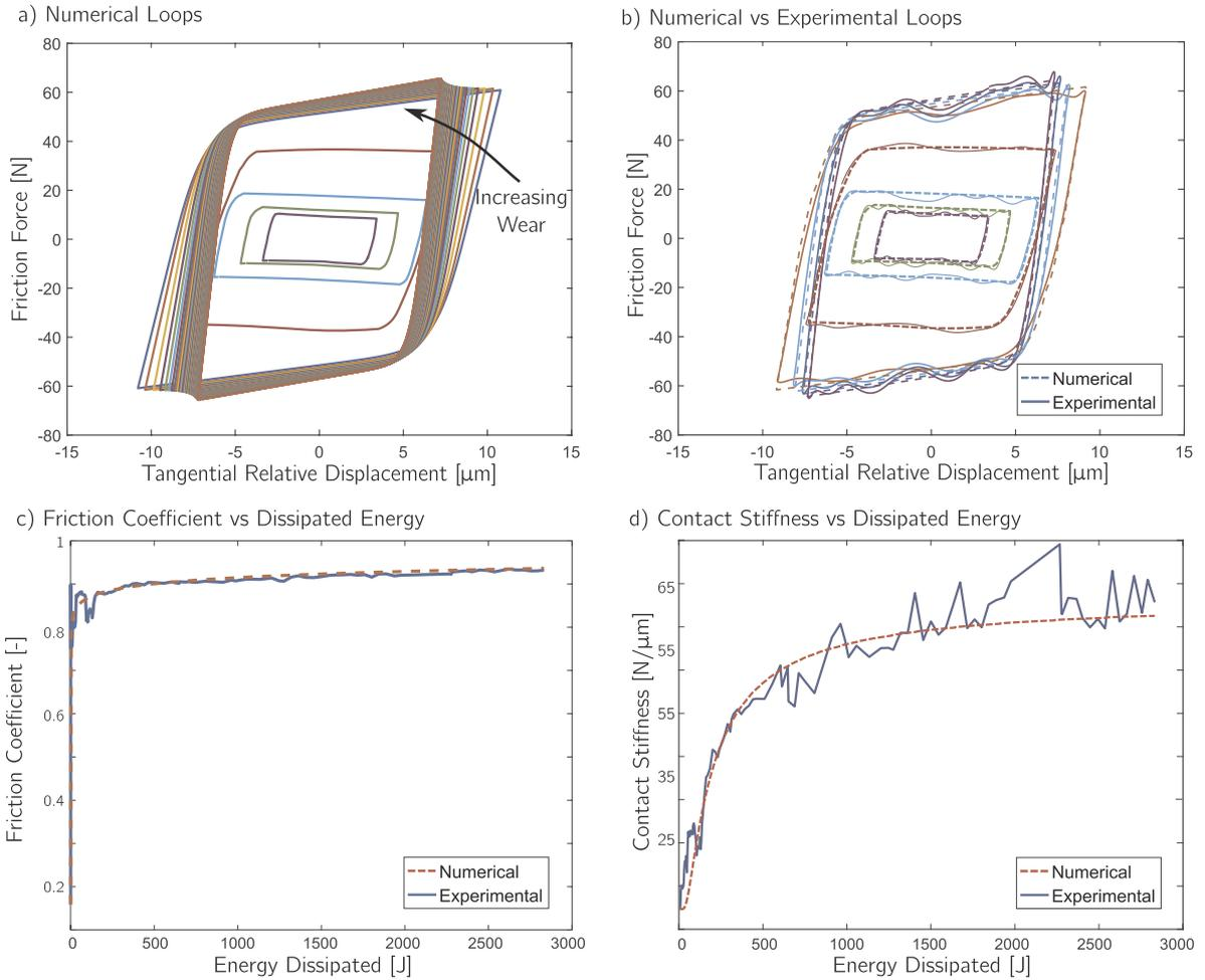
**Fig. 12.** Comparison between numerical and experimental results: a) numerical loops; b) numerical loops vs experimental loops for test 1; c) friction coefficient vs energy dissipated for test 1 (wear function defined in Table 3); d) contact stiffness vs energy dissipated for test 1 (wear function defined in Table 3).
