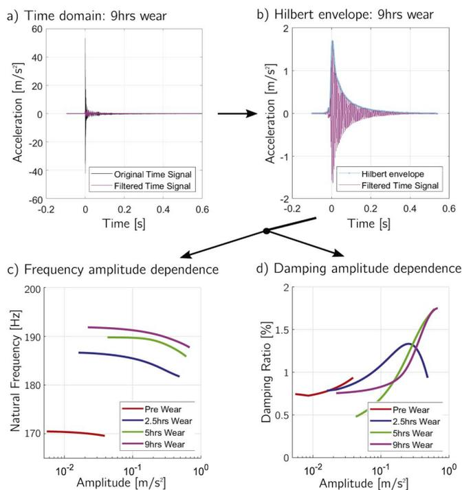
**Fig. 10.** Hilbert analysis to capture the evolution of the first natural frequency during test 5: a) Time signal at the end of the test; b) Hilbert envelope of the filtered signal; c-d) Amplitude dependencies of natural frequency and damping ratio obtained from the Hilbert envelopes.
