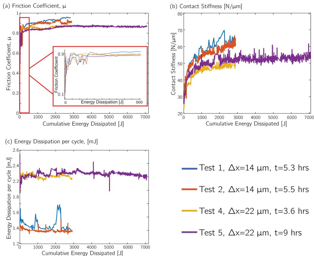
Fig. 5. Evolution of contact parameters with wear. Test conditions: excitation frequency = 100 Hz, normal load = 60 N, nominal area of contact =  $1\text{mm}^2$ , material = Stainless Steel, temperature =  $25^\circ\text{C}$ .
